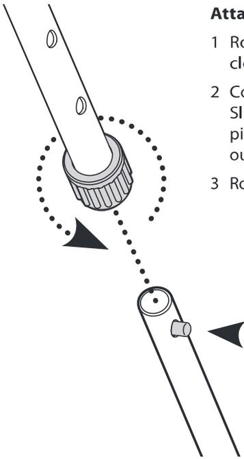
**Attaching the Upper Shaft to the Lower Shaft:**
