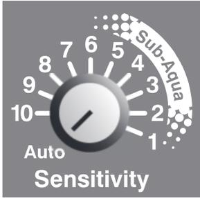
Sensitivity is the detector's level of response to its environment and to targets. The Sensitivity control allows you to adjust the level of sensitivity to suit the ground conditions in which you are detecting.
