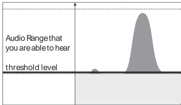
A threshold level that is too low does not allow faint target signals to be heard.
